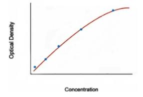
1. Any variation in operator, pipetting and washing technique, incubation time or temperature, and kit age can cause variation in result. Each user should obtain their own standard curve.
